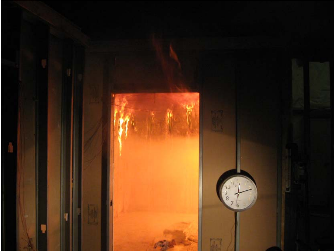
Flames exiting the doorway.
