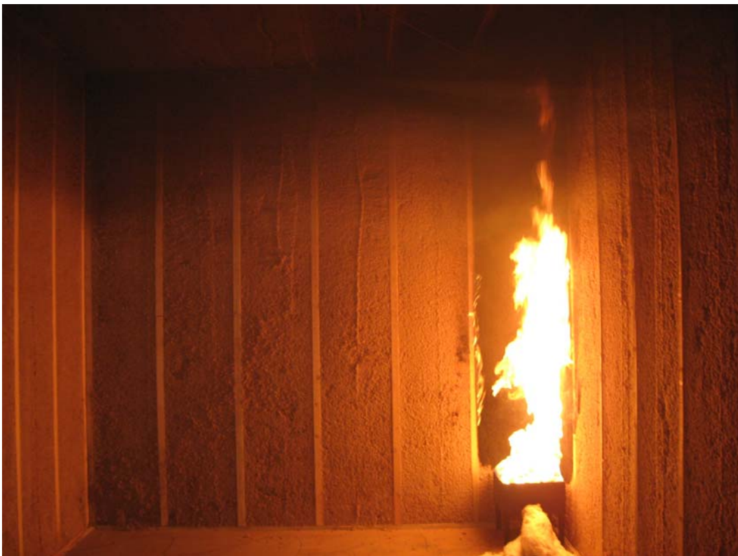
160 kW flame and ignition of studs.
